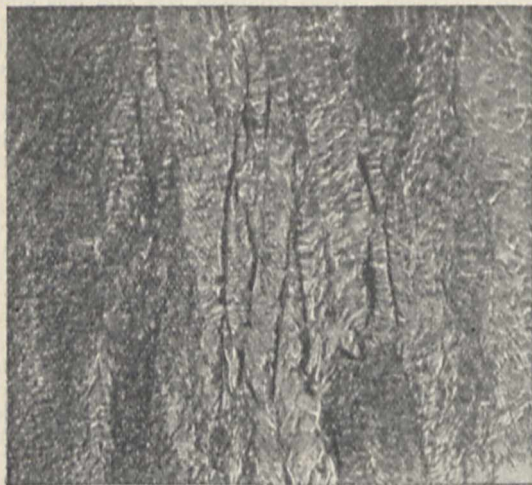
FIG. 1.—Hard-drawn gold wire. Magnification \times 700 .
