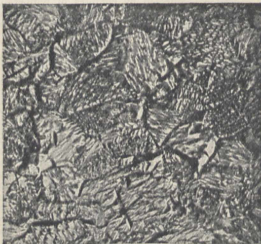
FIG. 2.—Hard-drawn gold wire after crystallisation at 280^{\circ} . Magnification \times 700 .
