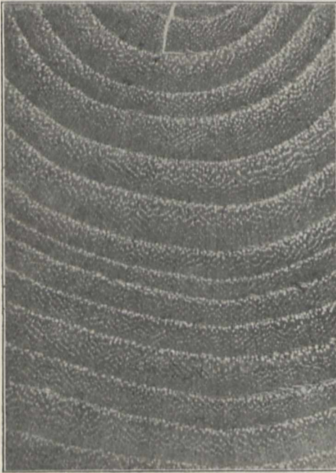
FIG. 2.—Common elm. Transverse section \times 33 .
