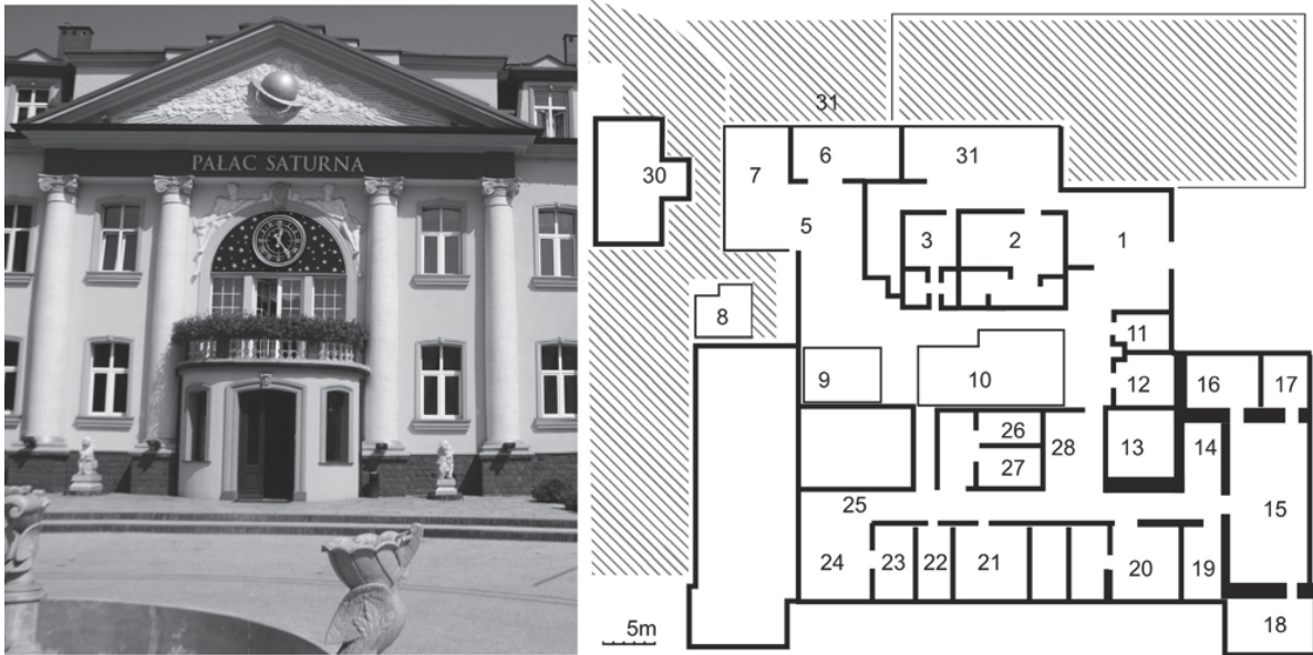
Fig. 4. Complex of Roman Thermae in Saturn's Palace in Czeladź; on the left – main entrance, on the right: functional program: 1 – Reception/main entrance, 2 – Apodyterion men's dressing rooms, toilet, shower, 3 – Apodyterion women's dressing rooms, toilet, shower, 4 – nudist beach, 5 – restaurant, 6 – rental, 7 – recreation deck, 8 – external swimming pool, 9 – swimming pool with massage chairs, 10 – swimming pool with waterstream, 11 – Temple of Sun solarium, 12 – Temple of Cleopatra bath and massage, 13 – Temple of water, 14 – Frigidarium cold water well, shower, 15 – atrium with ice fountain, 16 – Sauna of Cleopatra, 17 – biosauna, 18 – Sauna of Cesar, 19 – Laconium dry bath, 20 – Tepidarium rental, 21 – Calidarium thermal cave, 22 – Graduation Tower: thermal salt bath, 23 – Rasul, 24 – Hamam, 25 – Reception, 26 – Caldaria herbal bath, 27 – Caldaria flower bath, 28 – VIP Apodyterion dressing rooms, toilet shower, 29 – Beach, 30 – Temple of Saturn, 31 – Decks.
