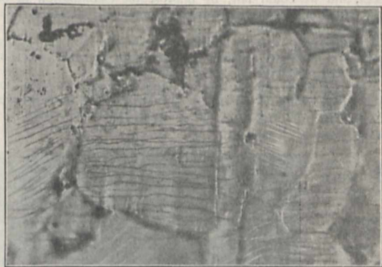
FIG. 1.—Soft sheet iron strained by tension. 400 diameters.
