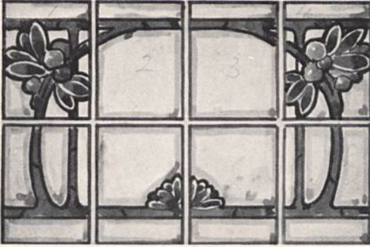
DOOR PANEL DIVIDED BY WOODEN BARS
