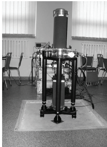
Fot. 8. Pomiar grawimetrem FG-5 na stanowisku WROCLAW Phot. 8. Measurement by FG-5 gravimeter at WROCLAW station
