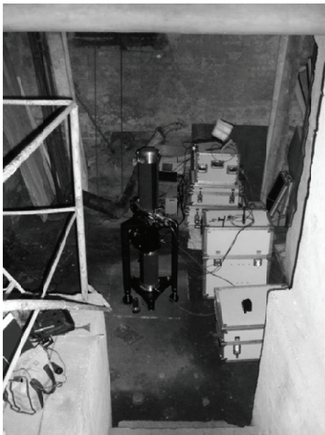
Fot. 7. Pomiar grawimetrem FG-5 na stanowisku JANOWICE Phot. 7. Measurement by FG-5 gravimeter at JANOWICE station
