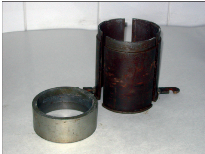
Phot. 7. Tripartite cylinder used for the forming of soil samples
