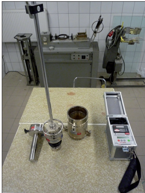
Phot. 8. Light drop-weight device ZFG for determining the Californian Bearing Ratio with dynamic method
