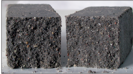
Phot. 3. View of the fractured sample after the test of bending strength
