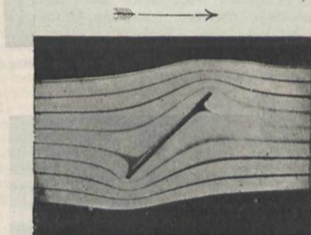
FIG. 8.—Inclined plate in thin sheet.
