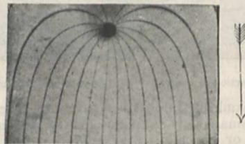
FIG. 7.—Uniform stream and "sink" in channel.
