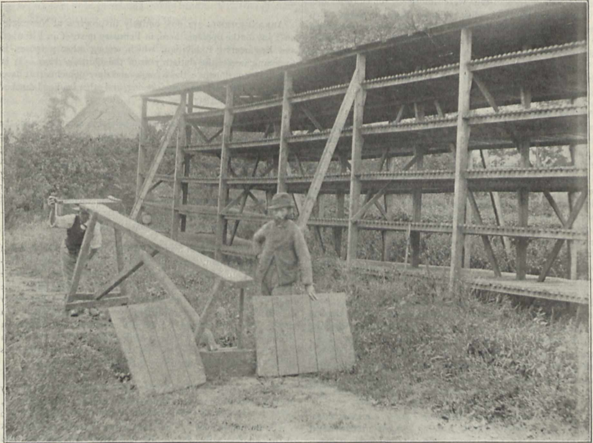
Woad Mill at Parson Drove. Two "balling-horses" are shown in front; between them is the "firm," from the further end of which a man is lifting one of the trays on which the balls are carried to the "ranges"; the latter are shown on the right
