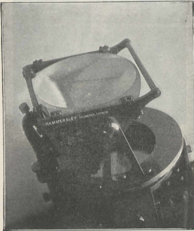
FIG. 9.—Details of objective prism.
