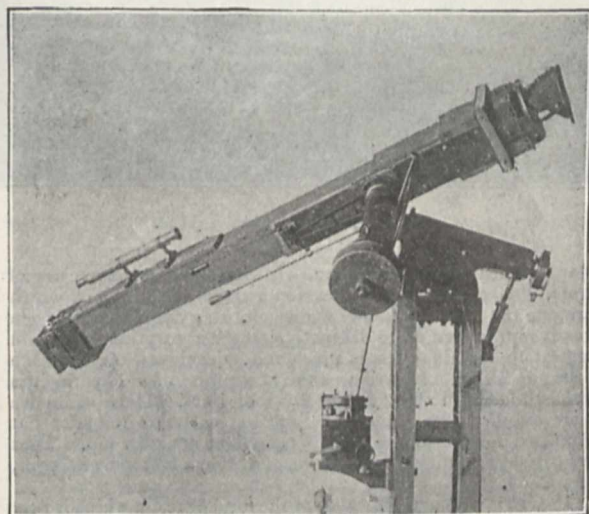
FIG. 8.—Showing method of photographing stellar spectra by the objective prism.
