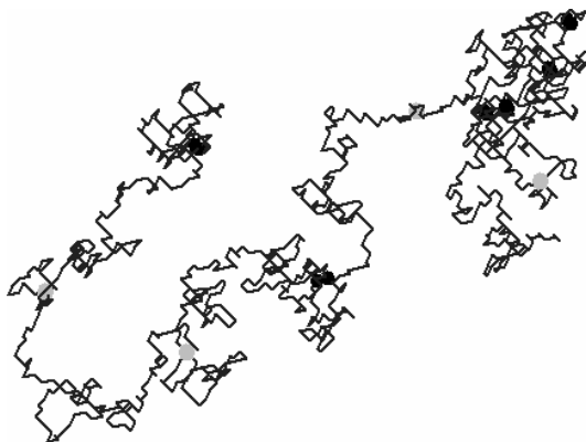
Fig. 1. Screenshot of a chain N = 1280 with Z_0 = 16 radicals during simulations. Grey circles mark radicals which have not recombined yet and black circles are the beads on which a radical has recombined forming cross-linking bonds and loops
