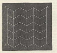
let the figure A B C D be bent round a hexagon, so as to form a hexagonal prism, the edges A B and C D being thus made to coincide. The prism will have open ends, and we have six rhombs left with which to close them, three for each end. Now bisect the prism by a plane perpendicular to its axis, and we shall have two typical bee cells.
