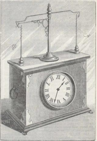
the principle of torsion. It has to be wound up daily, and the phase of the pendulum—that is to say, the time which elapses between two identical positions of the regulating system—is six seconds. The general mechanism does not differ from that of ordinary clocks; we find the main spring and other usual parts, and a train of wheels giving rotation to a vertical axis which is seen over the case and the rate of motion of which is to be regulated,
