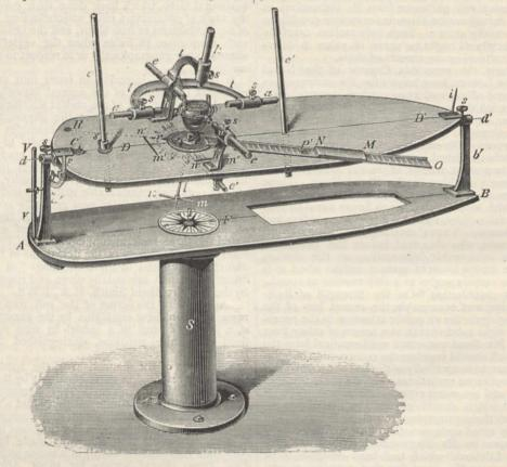
axis marked. At the point T, a compass-card is fixed to s, with its north and south points adjustable in the magnetic meridian.
