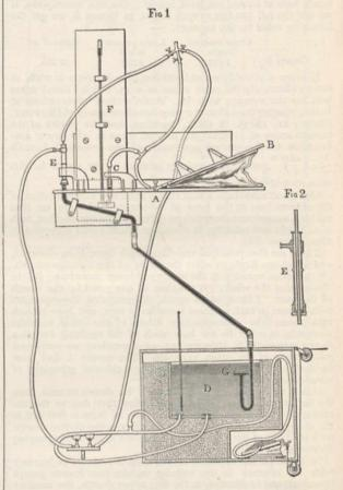
stirring was thus saturated with aqueous vapour, and did not cool the water in the bath by absorbing moisture from it. The nozzle of the bellows was connected to the U-shaped tube by a branch inserted just above the point where the gas-flame was applied. The air thus pumped through the upper part of the U-tube caused a rapid circulation of water through it. This method has the advantage of applying the heat in a manner which does not tend to make the water in one part of the bath
