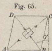
$$\operatorname{tg} DBC = \operatorname{tg} \left( 45^\circ + \frac{\gamma}{2} \right) = \frac{1/2 AC}{1/2 BD} = \frac{d + \Delta d}{d - \Delta d} = \frac{1 + \frac{\Delta d}{d}}{1 - \frac{\Delta d}{d}};$$
