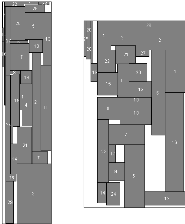
Fig. 2. Solutions received from Neuron-GIT algorithm, slicing instance on the left-90 Vofp, non-slicing on the right-76 Vofp.
