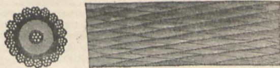
FIG. 34.—First Atlantic Cable, 1857 (natural size).
