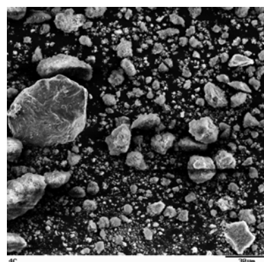
Fig. 6. Particle size distribution a) and SEM microphotograph b) of chromium(III) silicate (sample 4C)
