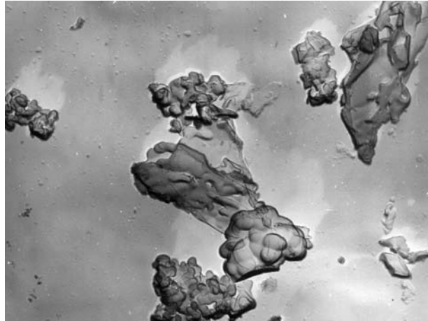
Fig. 3. TEM of raw silica following water extraction at 90-110 °C (~ 26,000x)
