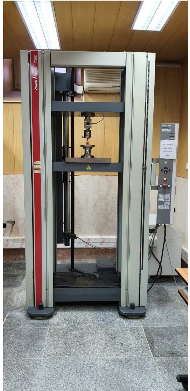
Fig. 2. Universal testing machine (UTM) (ZwickRoell ProLine Z050)
