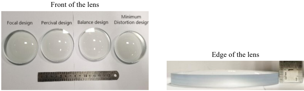
Fig. 6. Four groups of -8.00 D aspheric lenses physical picture obtained by the NSGA-II algorithm.
