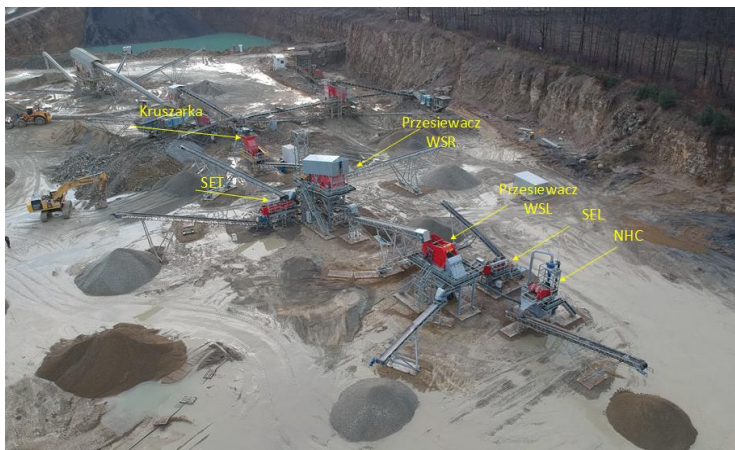
Rys. 1. Linia technologiczna w kopalni dolomitu Imielin, obraz z drona Fig. 1. Technological line in the Imielin dolomite mine, image from a drone
