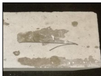
Rys. 2. Próbkę po badaniu wg AAR-3 z odbarwieniami, kwarcyt Fig. 2. Specimen with smears tested according to AAR-3, quartzite
