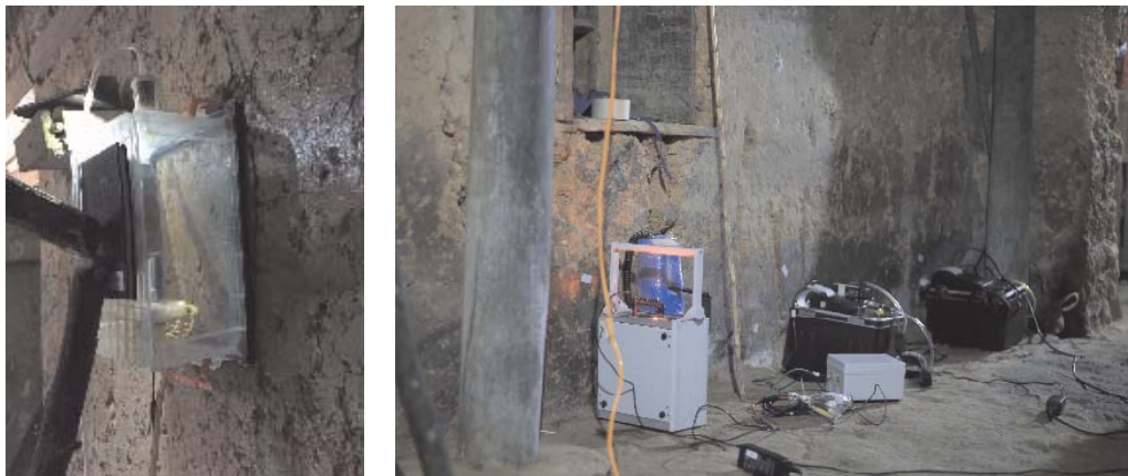
Fig. 2. Left : Measurement chamber with optional internal fan is pressed against wall to seal a defined volume of air in contact with a standardized surface area of mud; air is recirculated at 1 \text{ L min}^{-1} through instruments. Right : SARAD ® RTM2200 and two RAD7 units measuring radon and thoron during daytime in the room air of a northern Vietnamese mud house
