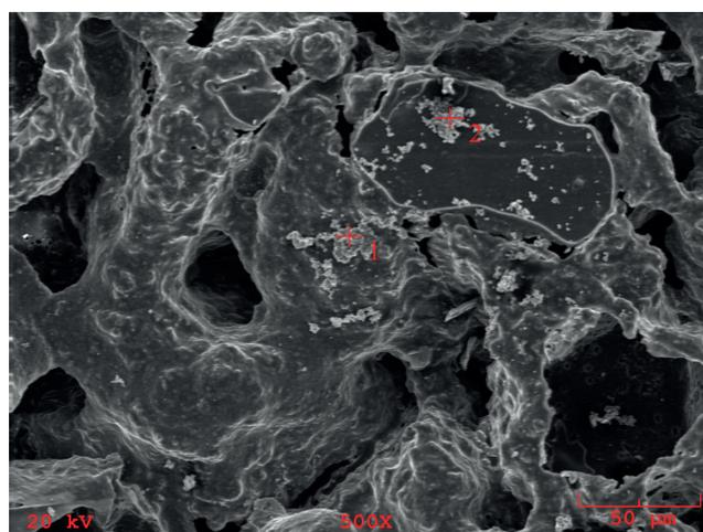
**Fig. 6.** Scanning electron microscopy (SEM) microphotographs of the PGS/HAp 80/20 scaffold after 14 days of incubation in simulated body fluid (SBF). The positions where energy dispersive spectroscopy (EDS) measurements took place are marked with red marks
