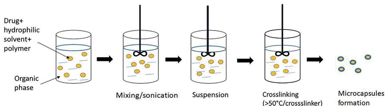
Fig. 2. Scheme for the use of the suspension crosslinking method to produce microcapsules
