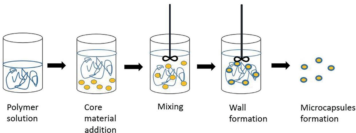
Fig. 6. Scheme for the use of the in situ polymerization method to produce microcapsules
