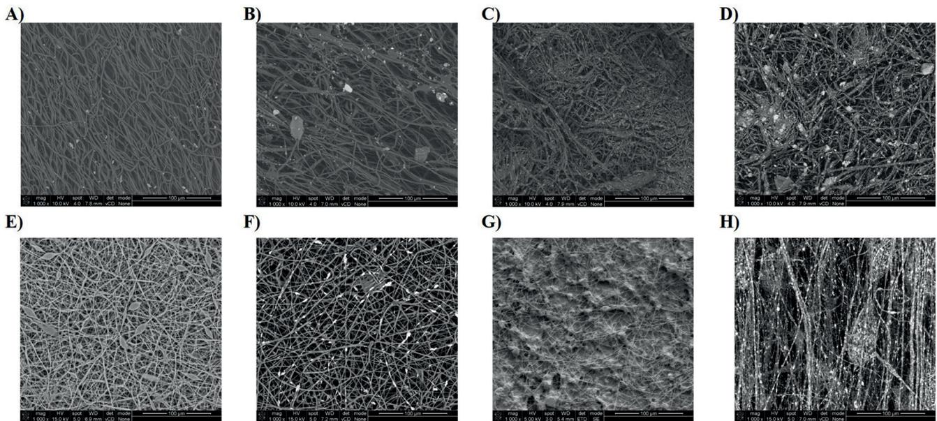
Fig. 1. Scanning electron microscopy (SEM) images of electrospun fibrous scaffolds. A. pure PCL; B. PCL\_HAP\_90/10; C. PCL\_HAP\_80/20; D. PCL\_HAP\_70/30; E. pure PLLA; F. PLLA\_HAP\_85/15; G. PLLA\_HAP\_75/25; H. PLLA\_HAP\_60/40
