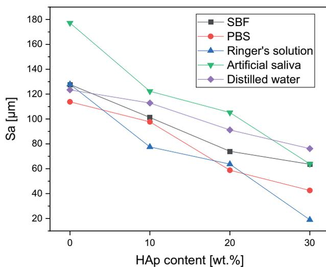
**Fig. 7.** Surface roughness of the reference and composite scaffolds after 2 week of incubation in simulated body fluid (SBF), phosphate buffered saline (PBS), Ringer's solution, artificial saliva, and distilled water. Roughness data was measured as an arithmetical mean height of the area (Sa) and showcased in the function of filler content
