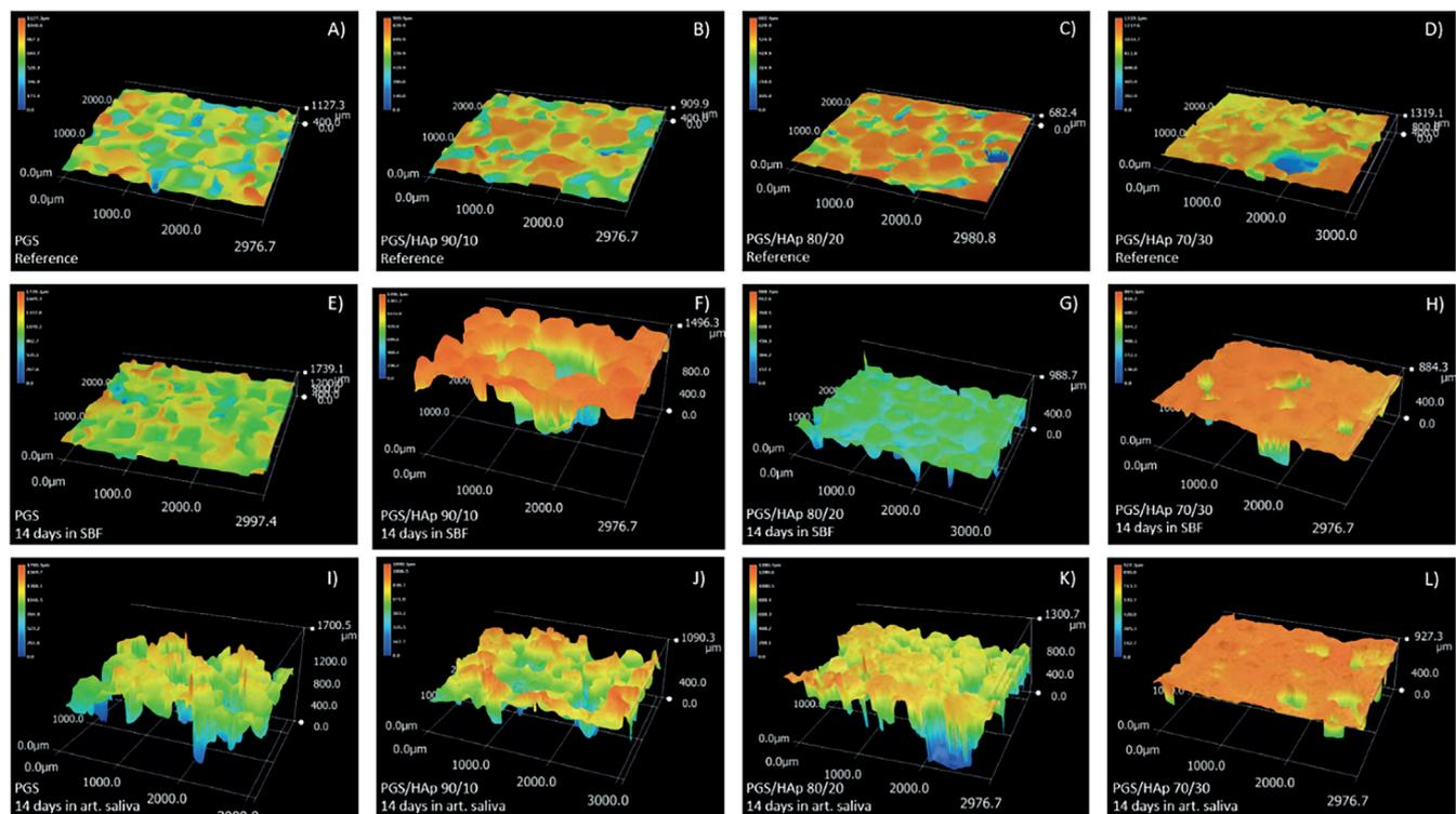
Fig. 10. Three-dimensional reconstructions of the surface of reference samples before incubation (A–D) as well as after 14 days of incubation in simulated body fluid (SBF) (E–H) and artificial saliva (I–L). The topography was obtained using reconstruction mode of optical microscope based on the pictures were taken with  $\times 100$  magnification
