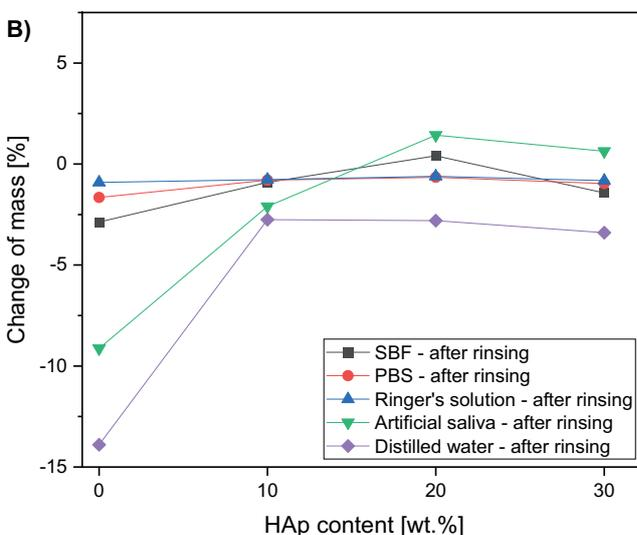
**Fig. 5.** Change in mass of the reference and composite scaffolds after 14 days incubation in simulated body fluid (SBF), phosphate buffered saline (PBS), Ringer's solution, artificial saliva, and distilled water for specimens dried straight after incubation (A) and samples dried followed by rinsing in distilled water in order to remove crystallized impurities (B)
