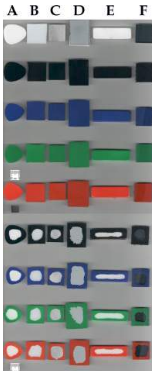
Figure 7. Complete set of samples used for the laboratory paint removal tests: (A) marble, (B) acrylic glass, (C) aluminum, (D) steel, (E) natural stone, (F) glass.
