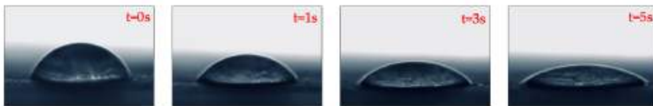
Figure S1. Dynamics of changes in the contact angle in the first phase of wetting of black graffiti paint coatings.
