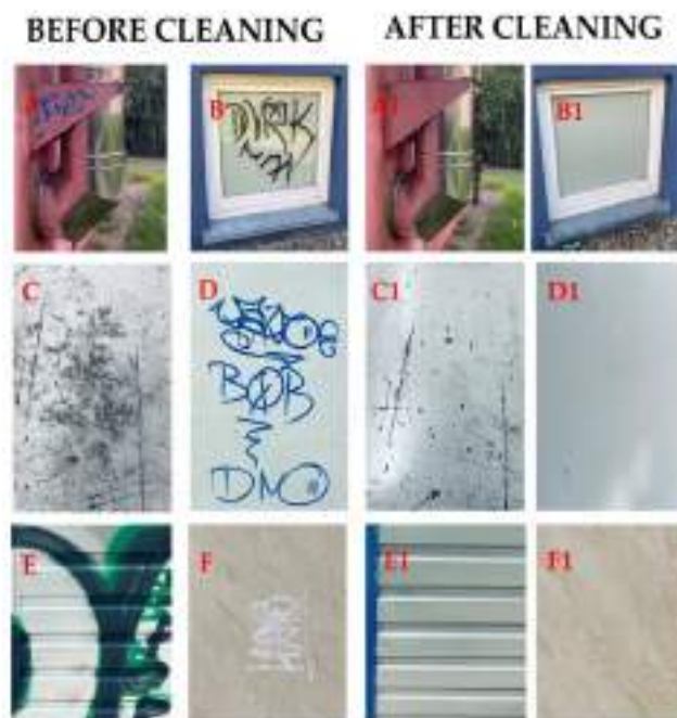
Figure 6. Different surfaces were cleaned with green nanostructured fluid no. 1 in the city of Wrocław: (A) stainless steel; (B) window glass; (C) concrete floor; (D) concrete floor with protective coating; (E) aluminum facade; (F) ceramic tiles.
