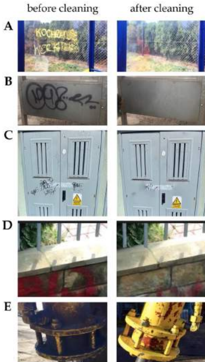
Figure 8. Different graffiti surfaces cleaned with eco-friendly graffiti remover MG-400-RO-20 in the city of Wrocław. (A). Glass surface at a bus stop. (B). Metal surface at a train stop. (C). Metal surface of a container. (D). Sandstone on a garden wall. (E). Metal surface of an excavator.
