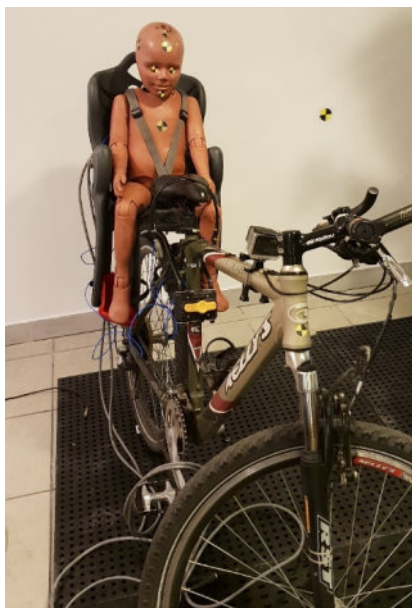
Fig. 32 Seated HybridIII-3YO ATD on the MTB with baby carrier
