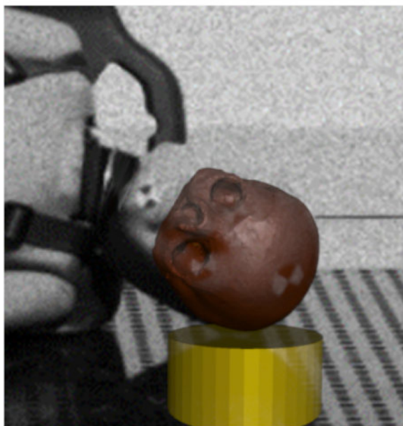
Fig. 53 Simulative case of a direct head impact to the ground with the presented aHEAD child model
