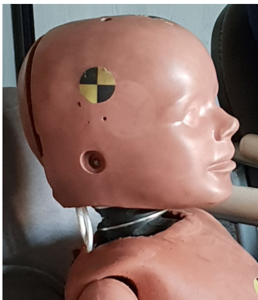
Fig. 40 Head and neck structure of the HybridIII-3YO dummy
