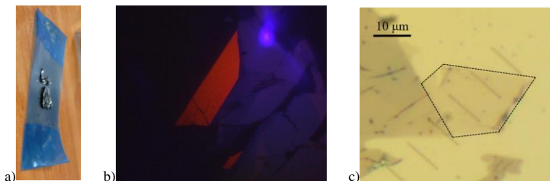
Fig. 1. a) Photograph of layered material on adhesive tape, b) micrograph of TMDs monolayer c) monolayer on GaAs nanomembranes substrate
