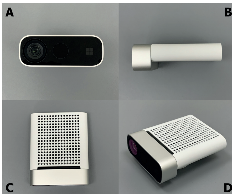
Fig. 2. Front view (A), lateral view (B), top view (C), and general view (D) of Microsoft Azure Kinect DK
