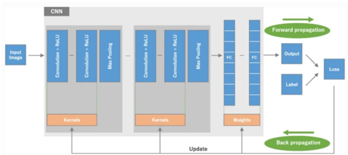
Figure 10. The training process of a CNN. In order to train a classification network we have to process through it hundreds, thousands or even millions of images and propagate loss (difference between expected and received output) back to adjust weights in each hidden layer. Source: (Liu et al. , 2015)
