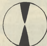
Zero point and its re- flected image as seen through the eyepiece.
