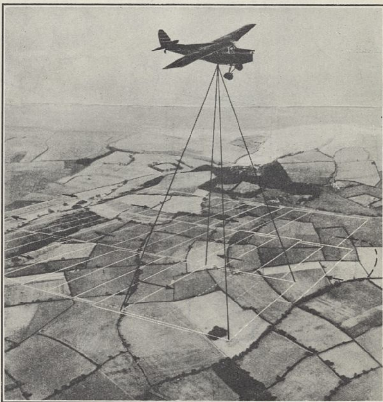
FIG. 1. Diagram illustrating how an aircraft covers the area to be photographed. By permission of Aerofilms, Ltd.
