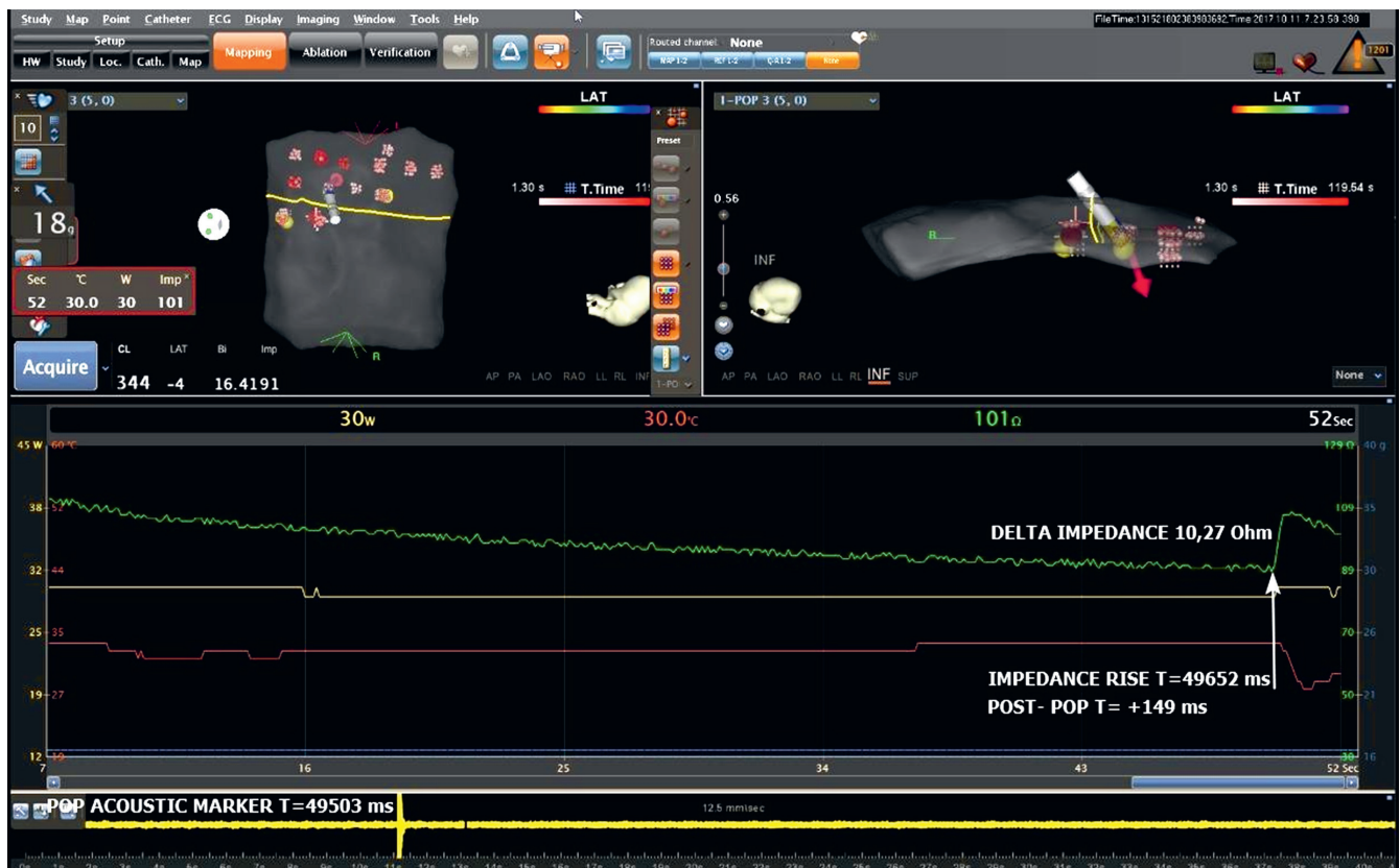
Fig. 2. Sample of measurements performed during experimental radiofrequency ablation (RFA). Acoustic marker T – steam pop occurrence time (data from the contact microphone connected to the electrophysiological system); delta impedance – the impedance rise value; impedance rise T – impedance abrupt rise time; post-pop T – steam pop and impedance rise time difference
