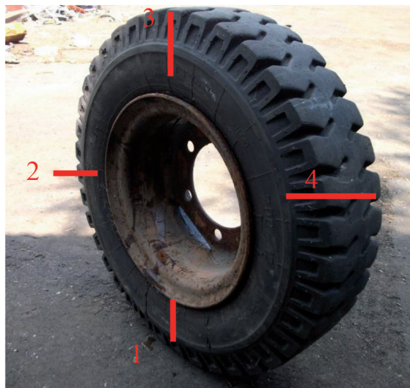
Fig. 6. Location of tread depth measuring points
