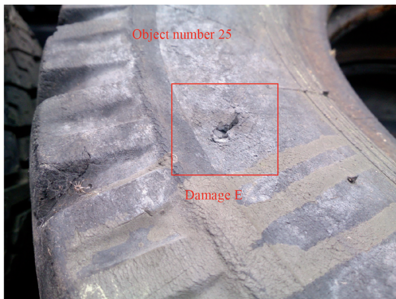
Fig. 13. Damage in object 25
