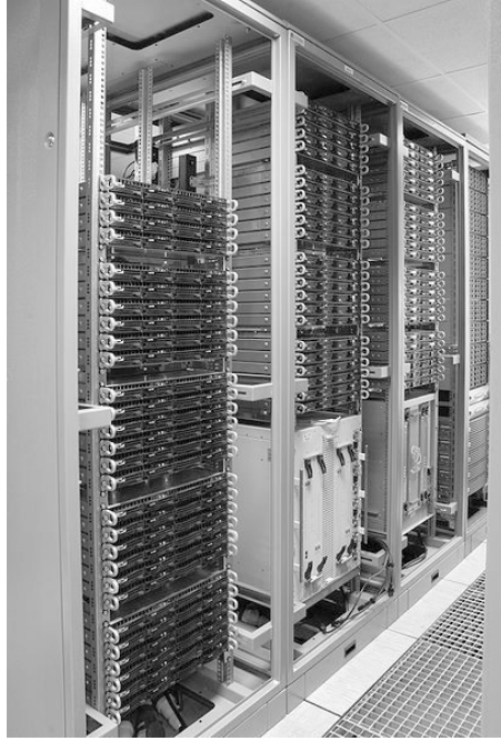
Fig. 1.6. The Nova cluster from the Wrocław Centre of Networking and Supercomputing, 2016 cores (19 TFLOPS). Source: WCNS [266].
